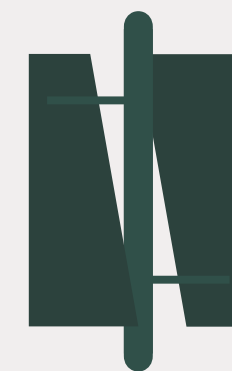
Figure 3. Basic design for vertical-axis turbine
